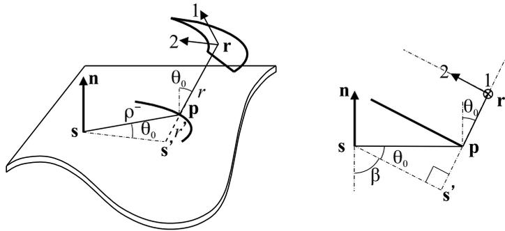
**Fig. 7.** Wavefronts for supersonic structural ray radiating acoustical rays. The acoustical wavefront at  $\mathbf{r}$  is a cone of axis  $\mathbf{n}$  with a straight generating line normal to the ray.
