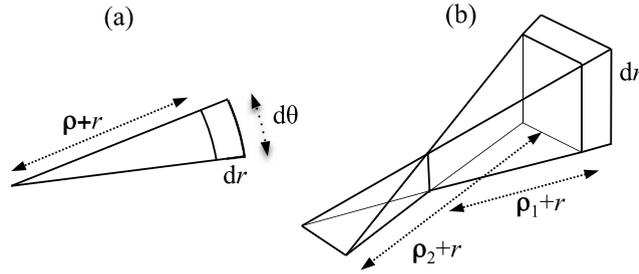
Fig. 5. Energy balance in a beam of rays, (a) in plate, (b) in fluid.
