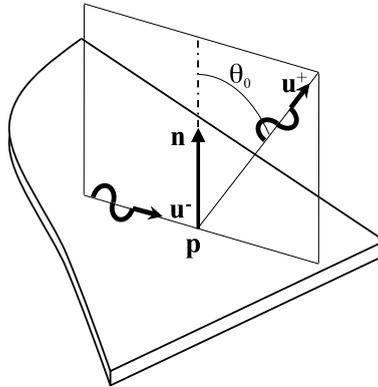
Fig. 2. Radiation of a supersonic structural ray, the acoustical ray starts with an emission angle  $\theta_0$  defined in Eq. (6).
