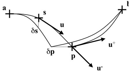
Fig. 1. Generalized Fermat's principle, the path **a**, **p**, **b** is stationary. The singular point **p** is constrained to lie on a surface, edge or vertex.
