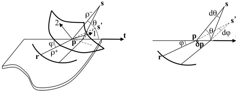
Fig. 10. Wavefronts for acoustical rays diffracted into structural rays by plate edges.
