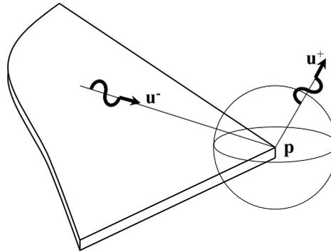
Fig. 4. Diffraction of a structural ray a corner, the acoustical ray may follow any direction.
