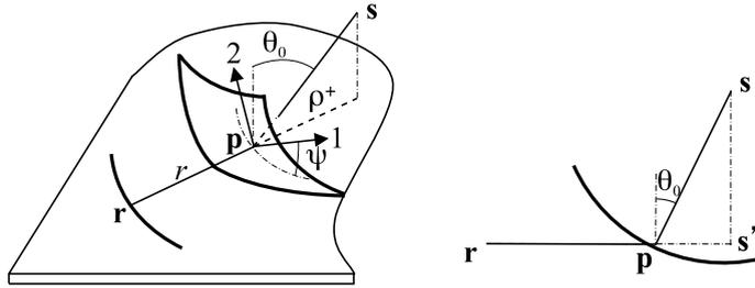
**Fig. 8.** Wavefronts for acoustical rays under incidence  $\theta_0$  converted into structural rays. The structural wavefront at  $\mathbf{p}$  is the curve intersection of the incident acoustical wavefront and the plate.
