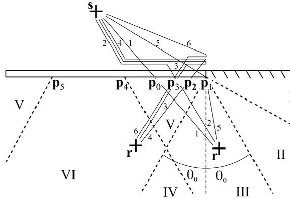
Fig. 12. Cylindrical wave hitting the plate. Six rays are transmitted through the plate and six zones numbered in Roman characters are defined depending on the number of rays reaching the zone.
