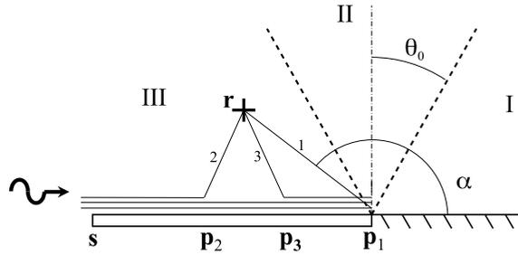
Fig. 11. Plane wave hitting the edge of a plate. Three rays are radiated towards the fluid and three zones numbered in Roman characters are defined depending on the number of rays reaching the zone.
