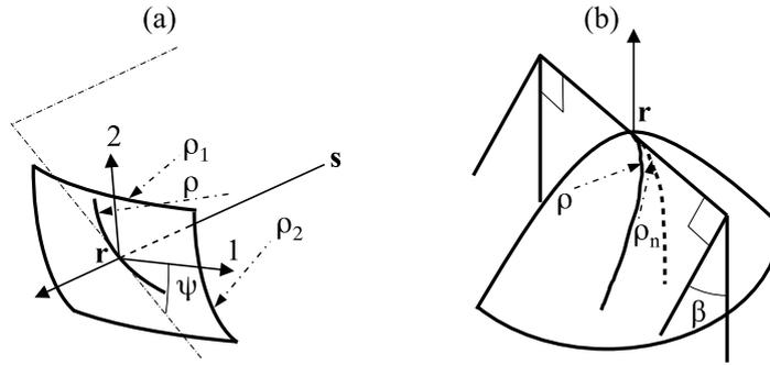
**Fig. 6.** Geometry of wavefront. (a) Euler's formula: 1 and 2 principal directions;  $\rho_1, \rho_2$  principal radii of curvature;  $\rho$  radius of curvature in a normal plane inclined by  $\psi$  to direction 1. (b): Meusnier's theorem:  $\rho_n$  radius of curvature in normal plane;  $\rho$  radius of curvature in a plane inclined by  $\beta$  to the normal plane.
