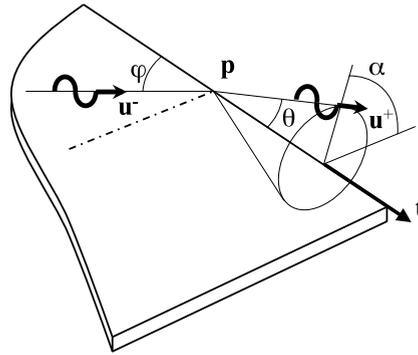
Fig. 3. Diffraction of a structural ray by edge, the acoustical ray lies in a Keller's cone which angle  $\theta$  is given in Eq. (7).
