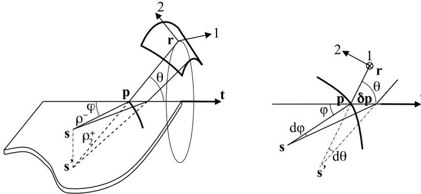
**Fig. 9.** Wavefronts for structural rays diffracted by edges. The acoustical wavefront at  $\mathbf{r}$  is a cone of axis  $\mathbf{t}$  with a curved generating line.
