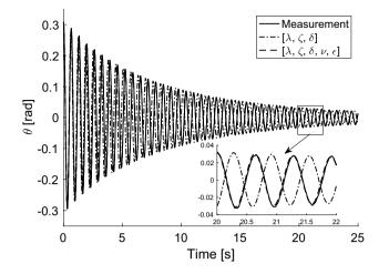
**Fig. 7** Time evolution of  $\theta$  for a PDMS-sphere/glass-plate torsional contact. Solid line: measurement. Dash-dot line: solution to Eq. (1) with  $\lambda$ ,  $\zeta$ , and  $\delta$ . Dashed line: with  $\lambda$ ,  $\zeta$ ,  $\delta$ ,  $\nu$ , and  $\epsilon$
