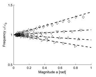
**Fig. 3** Evolution of frequency with amplitude for a pure quadratic dissipative force  $\delta \dot{\theta}^2 \operatorname{sgn}(\dot{\theta})/\omega_0^2$ . Symbols: numerical solution to Eq. (1) with initial conditions  $\theta(0) = 1$ ,  $\dot{\theta}(0) = 0$  (one value per half-period) with  $\delta = 0.05$  (>), 0.1 ( $\Delta$ ), 0.3 ( $\nabla$ ) or 0.8 ( $\Diamond$ ). Broken line: Eq. (9)
