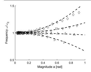
**Fig. 5** Evolution of frequency with amplitude for a pure cubic elastic force  $\epsilon\theta^3$ ). Symbols: numerical solution to Eq. (1) with initial conditions  $\theta(0) = 1$ ,  $\dot{\theta}(0) = 0$  (one value per half-period) with  $\zeta = 0.05$  and  $\epsilon = -0.9$  ( $\triangleright$ ), -0.1 ( $\Delta$ ), 0.5 ( $\nabla$ ), 1.5 ( $\Diamond$ ). Broken lines: Eq. (9)
