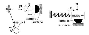
**Fig.1** Left: principle of a torsional pendulum with a sphere/plane contact at the extremity of the rotation axis. Right: principle of a translational oscillator with a sphere in contact with a plane and attached to the moving mass
