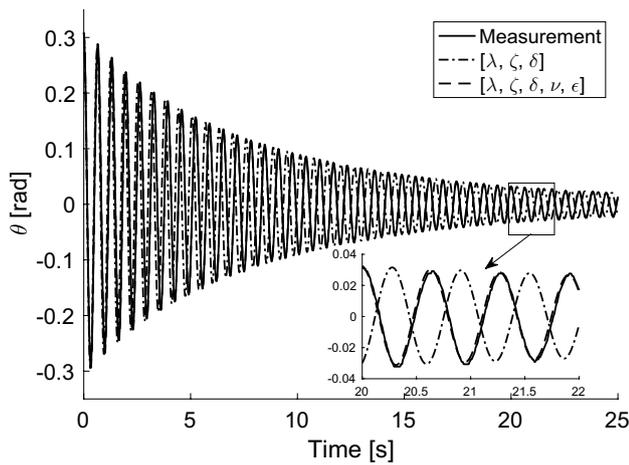
**Fig. 7** Time evolution of  $\theta$  for a PDMS-sphere/glass-plate torsional contact. Solid line: measurement. Dash-dot line: solution to Eq. (1) with  $\lambda$ ,  $\zeta$ , and  $\delta$ . Dashed line: with  $\lambda$ ,  $\zeta$ ,  $\delta$ ,  $\nu$ , and  $\epsilon$
