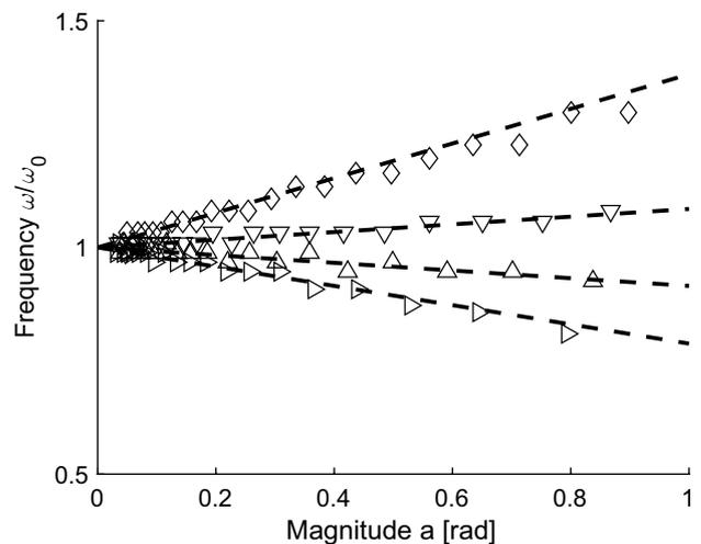
**Fig. 4** Evolution of frequency with amplitude for a pure quadratic elastic force  $v\theta^2\text{sgn}(\theta)$ . Symbols: numerical solution to Eq. (1) with initial conditions  $\theta(0) = 1, \dot{\theta}(0) = 0$  (one value per half-period) with  $\zeta = 0.05$  and  $v = -0.5$  ( $\triangleright$ ),  $-0.2$  ( $\triangle$ ),  $0.2$  ( $\nabla$ ),  $0.9$  ( $\diamond$ ). Broken lines: Eq. (9)
