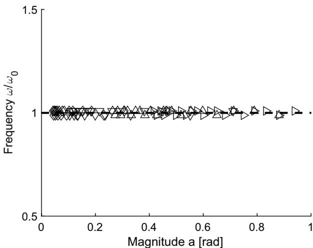
**Fig. 3** Evolution of frequency with amplitude for a pure quadratic dissipative force  $\delta\dot{\theta}^2\text{sgn}(\dot{\theta})/\omega_0^2$ . Symbols: numerical solution to Eq. (1) with initial conditions  $\theta(0) = 1, \dot{\theta}(0) = 0$  (one value per half-period) with  $\delta = 0.05$  ( $\triangleright$ ),  $0.1$  ( $\triangle$ ),  $0.3$  ( $\nabla$ ) or  $0.8$  ( $\diamond$ ). Broken line: Eq. (9)
