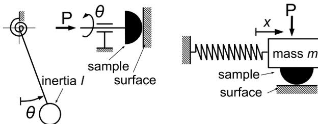
**Fig. 1** Left: principle of a torsional pendulum with a sphere/plane contact at the extremity of the rotation axis. Right: principle of a translational oscillator with a sphere in contact with a plane and attached to the moving mass
