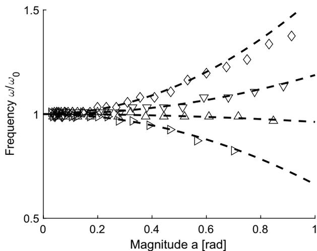
**Fig. 5** Evolution of frequency with amplitude for a pure cubic elastic force  $\epsilon\theta^3$ ). Symbols: numerical solution to Eq. (1) with initial conditions  $\theta(0) = 1, \dot{\theta}(0) = 0$  (one value per half-period) with  $\zeta = 0.05$  and  $\epsilon = -0.9$  ( $\triangleright$ ),  $-0.1$  ( $\triangle$ ),  $0.5$  ( $\nabla$ ),  $1.5$  ( $\diamond$ ). Broken lines: Eq. (9)
